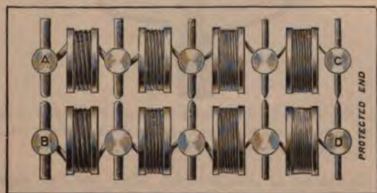
Fig. 81. DIAGRAM OF DOUBLE FORM OF GUARD FOR INSTRUMENTS.
